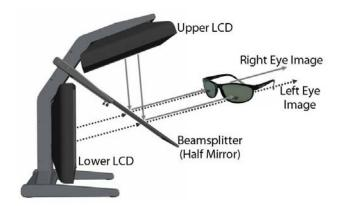
Operating principle of the StereoMirror monitor
